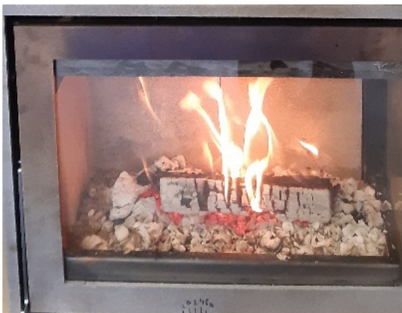
Picture 1 Positioning of the wood during the nominal tests
